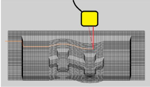
FIGURE 2. Concept of a surface scan, using a target model from ref.[3].
