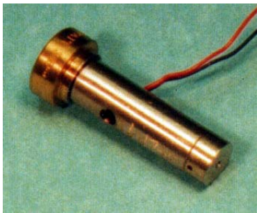
Figure 4 Single channel drop-on-demand dispensing device; T < 240^{\circ}\text{C} .
