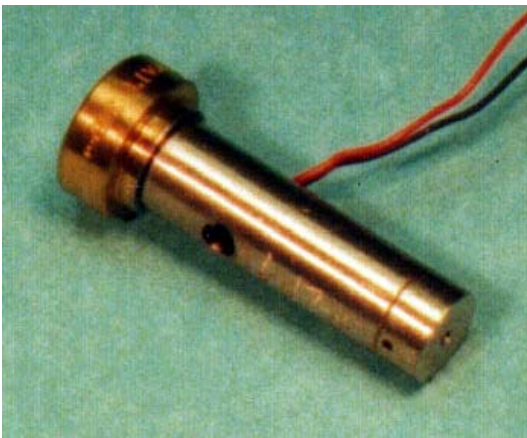
Figure 5 Single-jet, high-temp printhead (6-mm diameter)
