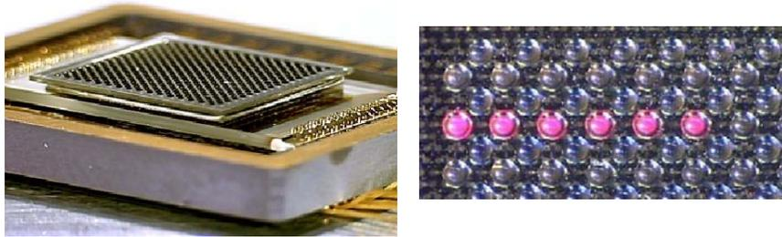
Fig. 4. Smart pixel array module (left) and printed 250 μm diameter microlens array in module with VCSELs under 6 lenslet turned on (right). (Photos courtesy of Y. Liu & A. Cox of Honeywell.)
