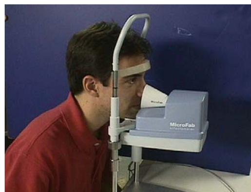
Figure 5: Piezo-micro-dispensing olfactometer.
