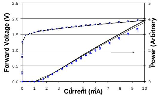
**Figure 12.** DC characteristics of VCSELs: solid curves – before solder bonding; cross marks – after solder bonding.
