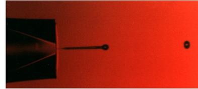
Figure 1. Dispensing of 50  $\mu\text{m}$  ethylene glycol drops at 2 kHz.
