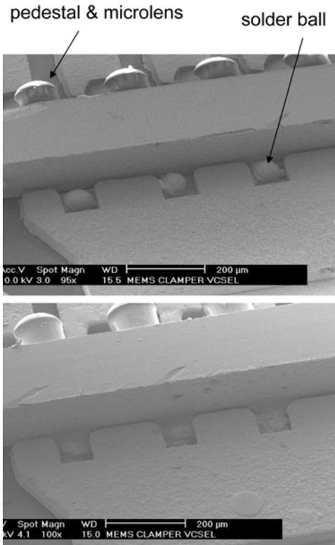
**Figure 11.** Solder balls interconnect cathode of VCSEL array die with Au-plated copper pad, before re-flow (top) and after re-flow (bottom).
