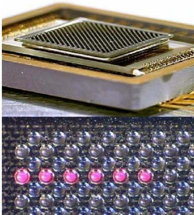
**Figure 5.** Smart pixel array module (top) and printed  $250\mu\text{m}$  diameter microlens array in module with VCSELs under. 6 VCSELs are turned on (bottom). (Photo courtesy of Honeywell)
