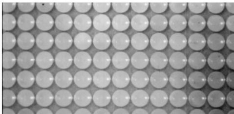
**Figure 4.** Printed microlens array of diameter  $916\mu\text{m}$  on  $1\text{ mm}$  centers with focal lengths of  $1.10\pm 0.01\text{ mm}$ .
