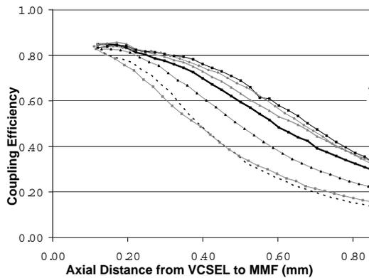
**Figure 7.** Coupling efficiency from VCSEL to MMF for different epoxy drop number  $N$  printed on pedestals to form microlenses. Parameters are given in the text.
