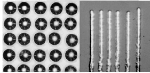
**Figure 9.**  $24\mu\text{m}$  diameter solder bumps on  $35\mu\text{m}$  centers (left), and an array of  $24\mu\text{m}$  towers (right).
