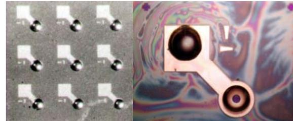
**Figure 10.** VCSEL array with printed  $90\mu\text{m}$  microlenses on emitters (left); VCSEL with microlens on emitter and  $60\mu\text{m}$  solder bump on bonding pad (right).
