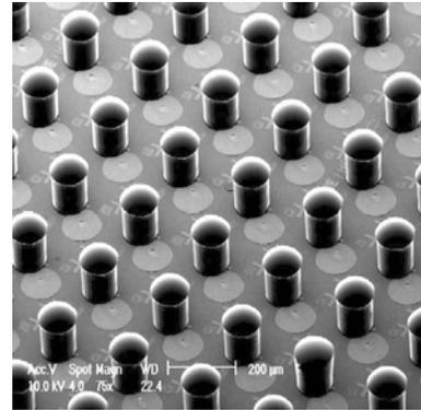
**Figure 6.** Pedestal-microlens structure fabricated on VCSEL wafer.
