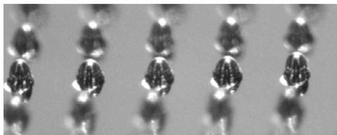
**Figure 8.**  $100\mu\text{m}$  diameter solder bumps placed onto  $100\mu\text{m}$  pads on  $250\mu\text{m}$  centers at 400 per second.
