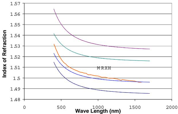
**Figure 3.** Dispersion curves of refractive indices of optical polymers, including optical epoxy MRXH.
