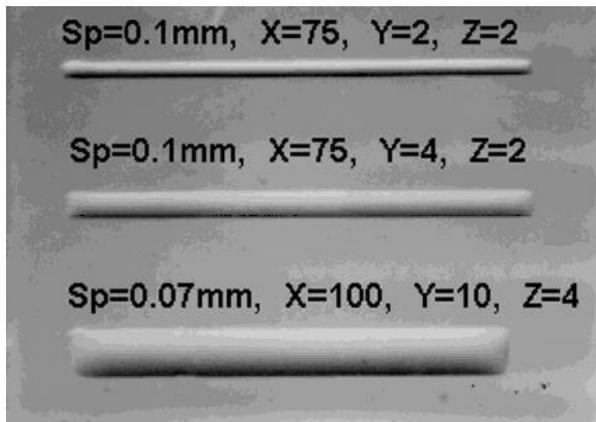
**Figure 7.** Printed bond lines (top is 300 $\mu$ m wide) made by deposition at 125EC of 60 $\mu$ m droplets of thermoset epoxy, where site spacings ( $Sp$ ), number of sites in horizontal ( $X$ ) & vertical ( $Y$ ) directions in substrate plane and number of droplets per site ( $Z$ ) are as indicated.
