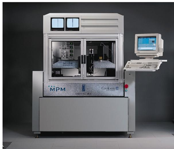
Figure 4. MPM demand-mode solder printing (Metal-Jet®) demonstration platform.
