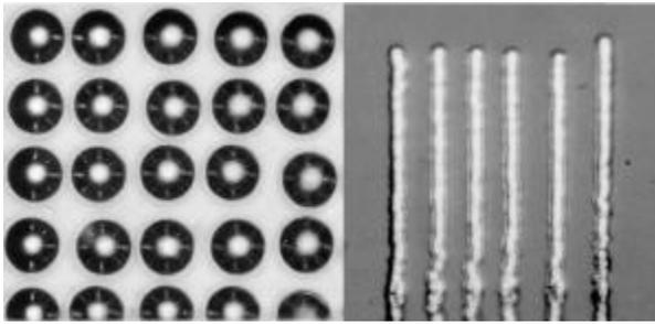
Figure 2. Printed array of 24  $\mu\text{m}$  diameter solder bumps (left) and 25  $\mu\text{m}$  wide, 400  $\mu\text{m}$  high solder towers (right).
