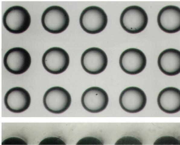
**Figure 5.** Array of 95  $\mu\text{m}$  diameter, 34  $\mu\text{m}$  high, printed microlenses (spacer bumps), in substrate plane (top) and in profile (bottom).
