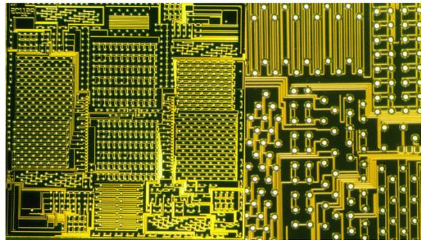
Figure 3. Portions of microprocessor test vehicle with 1,440 printed with 60  $\mu\text{m}$  solder droplets at 100% yield.
