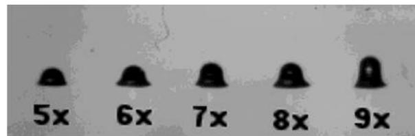
**Figure 6.** Increasing printed epoxy spacer-bump / microlens height by UV-flash after each of the indicated total number of 50 $\mu\text{m}$  droplets.
