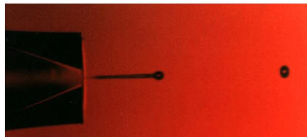
Figure 1. Generation of 50  $\mu\text{m}$  droplets by DOD microjet at 2 kHz.
