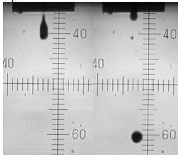
**Figure 6:** The drop formation process for the same Solder Jet device shown in the previous figure, but using a different drive waveform. The drop rate is 120 Hz and drop size is 106µm.
