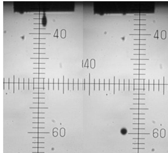
**Figure 5:** The drop formation process for a Solder Jet device is shown at two times during the process. The drop rate is 120 Hz and drop size is 62µm.
