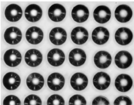
Figure 8:  $25\mu\text{m}$  bumps of  $63/37$  deposited on  $35\mu\text{m}$  pitch using Solder Jet Technology.
