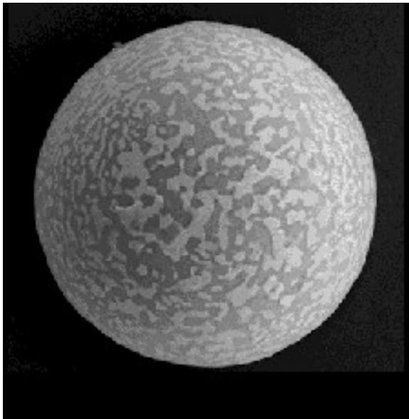
**Figure 3:** SEM of the top of a 60µm diameter 63/37 bump deposited onto the IC test vehicle.
