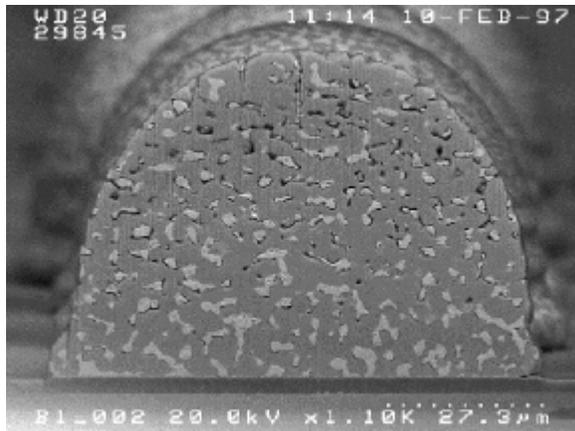
**Figure 4:** Cross-section of bump shown in previous figure.
