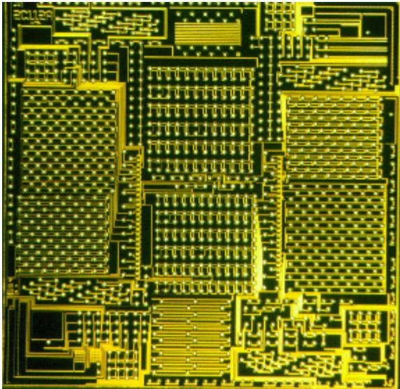
**Figure 1:** IC test vehicle with 1440 pads, bumped with 63/37 using Solder Jet Technology. Ball size is 70 $\mu$ m.
