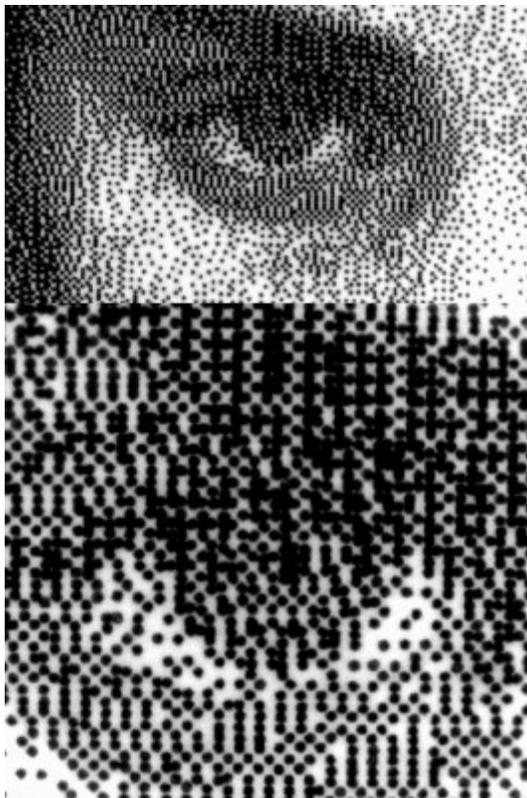
*Figure 4: Photomicrograph of fixed spot printing using the same printhead and original image as was used in Figure 5.*
