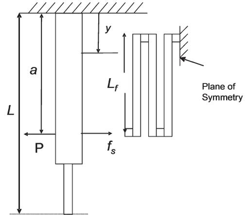
Fig. 7. Approximated model of a type-1 micro clasper used for the analytical calculation.
