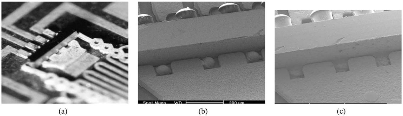
Fig. 15. Backside view of a  $4 \times 1$  VCSEL array held by a micro clasper (a) before solder printing, (b) after printing, and (c) after reflow.
