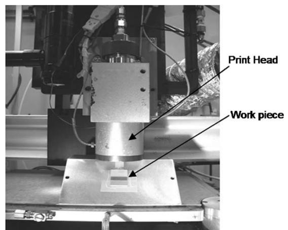
Fig. 13. Solder-jet head used for solder printing.
