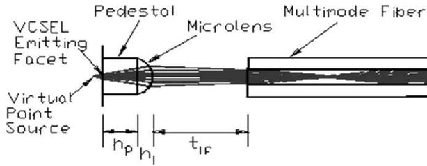
Fig. 1. Concept of the integration of a microoptic element (pedestal and microlens) with a VCSEL for effective light coupling to an MMF.
