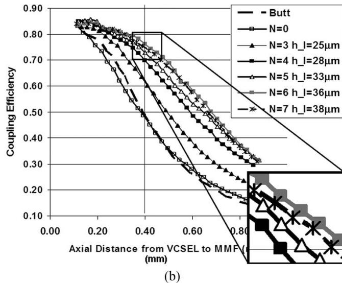
Fig. 4. (a) Measured dc characteristics of VCSELs. (b) Measured coupling efficiency versus axial distance (from the VCSEL emitting facet to the MMF tip) for different lens heights with a pedestal height of 100 μm and a diameter of 120 μm.
