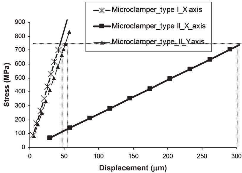
Fig. 10. Von Mises stresses in the arms of the springs with varying tip displacements. Corresponding displacements are marked out for a yield stress of 750 MPa.
