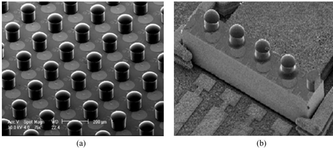
Fig. 3. SEM photomicrographs. (a) Wafer-level fabricated microoptic element array and (b) diced 4 × 1 VCSEL array.
