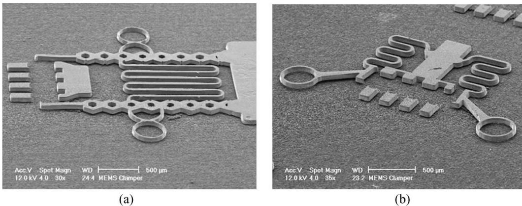
Fig. 11. SEM pictures. (a) Type-1 micro clamper structure. (b) Type-2 micro clamper structure.
