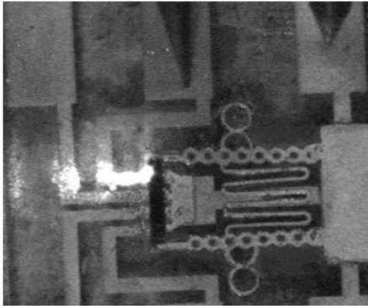
Fig. 16. Fully assembled VCSEL array with one of the VCSELs fired on and emitting 850-nm laser as seen by an infrared-sensitive camera.
