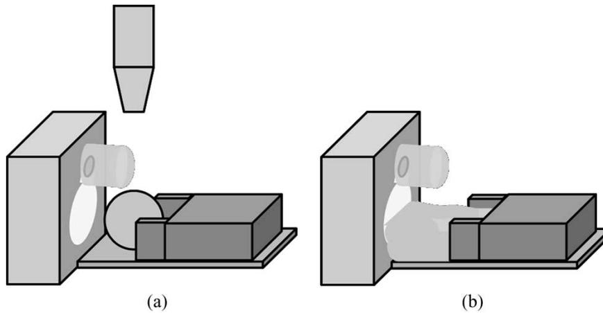
Fig. 14. Schematic diagrams. (a) Solder ball printed into the micromold structure. (b) Electrical interconnection established after reflow.
