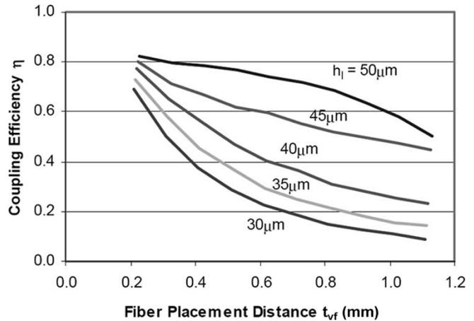
Fig. 2. Coupling efficiency versus axial distance (from the VCSEL emitting facet to the MMF tip) for different lens heights with a pedestal height of 80  $\mu\text{m}$  and a diameter of 120  $\mu\text{m}$ .
