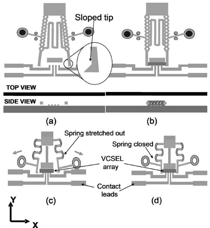
Fig. 5. Mechanical assembly procedures for (a), (b) the type-1 and (c), (d) the type-2 micro clampers.
