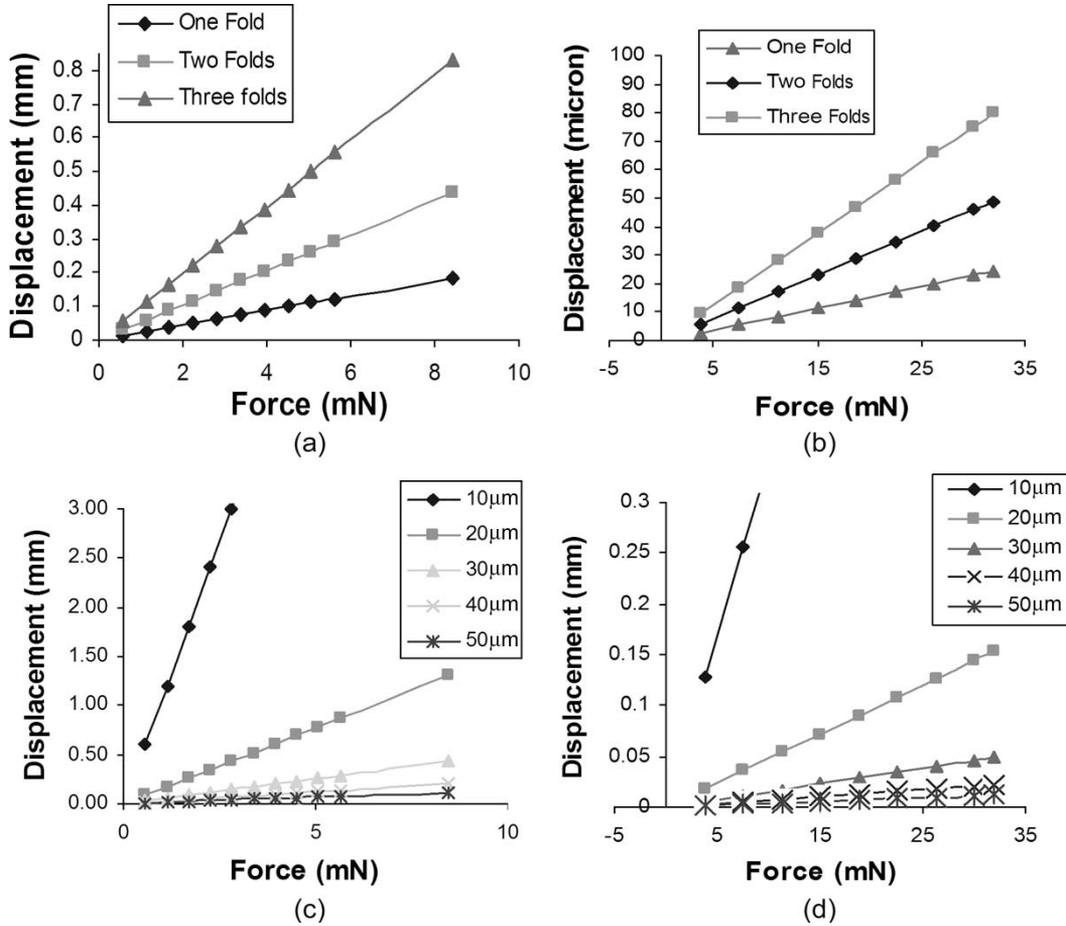
Fig. 9. Type-2 micro-clamper clamping forces with varying parameters. (a) Variation of the spring constant in the  $x$ -direction with varying numbers of folds. (b) Variation of the spring constant in  $y$ -direction with varying numbers of folds. (c) Variation of the spring constant in the  $x$ -direction with varying widths of beams. (d) Variation of the spring constant in  $y$ -direction with varying widths of beams.
