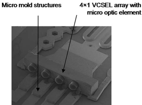
Fig. 12. A 4 × 1 VCSEL array held in position by a type-1 micro clamper.
