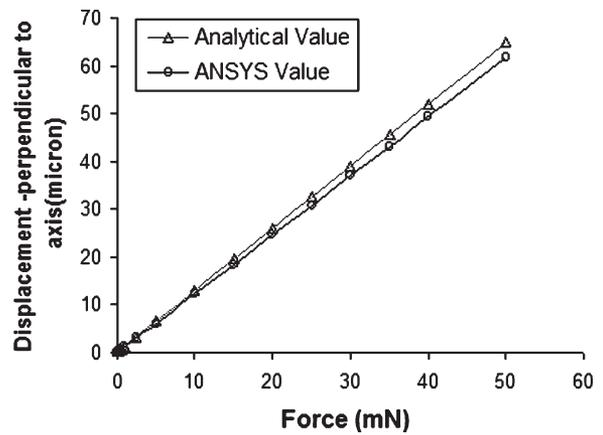
Fig. 8. Comparison of analytical and ANSYS values for the deflection of the clasper arm in the  $x$ -direction of the type-1 micro clasper.
