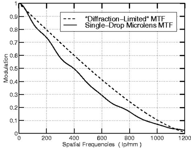
**Figure 4.** Modulation transfer function for an f/1.25 microlens printed with one 50 $\mu\text{m}$  drop of UV-curing optical material (solid curve), compared to ideal, diffraction-limited case (dashed curve) at same f/#.
