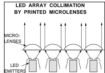
**Figure 6.** Geometry for LED array collimation by printed microlenses.
