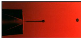
**Figure 1.** Generation of 50 $\mu\text{m}$  droplets at 2 kHz.
