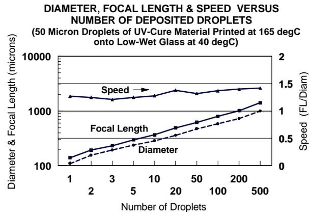
**Figure 3.** Variation of printed hemispherical microlens geometry with number of deposited droplets.
