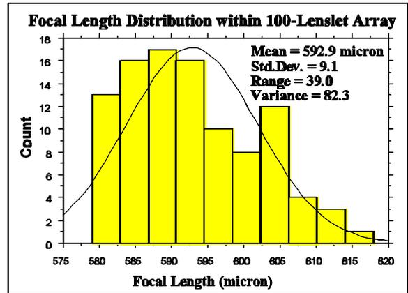
**Figure 5.** Distribution of focal lengths of 100 each 0.5  $\mu\text{m}$  diameter microlenses printed in 10x10 array on 750  $\mu\text{m}$  centers, showing a typical standard deviation from the average value of 1.5%.
