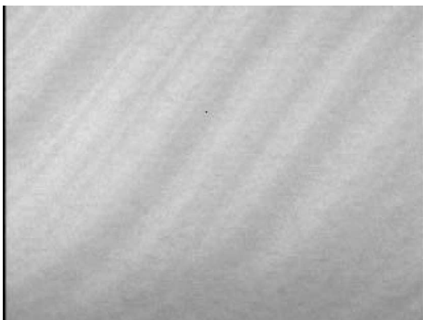
Fig.10 A portion of PPV-PCBM film on ITO/glass at 45°C ; spot pitch 110µm each in X and Y
