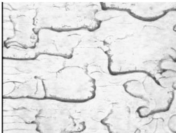
Fig.12 A portion of PPV-PCBM film on ITO/glass at 45°C ; spot pitch 80µm each in X and Y
