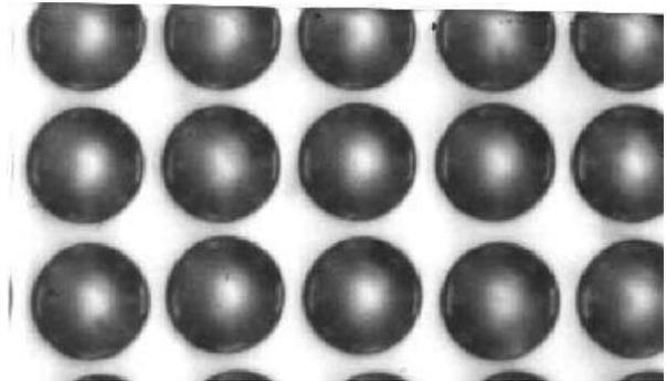
**Figure 4: Pictures an array of 40 $\mu$ m diameter micro-lenses printed on 50 $\mu$ m centers.**
