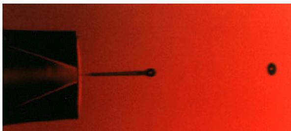
*Figure 1: Generation of 50  $\mu\text{m}$  drops by a DOD print head at 2 kHz.*
