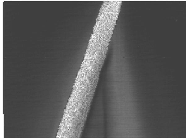
**Figure 8:** SEM of ink jet printed  $Zn_2SiO_4:Mn$  phosphor powder 90µm line.
