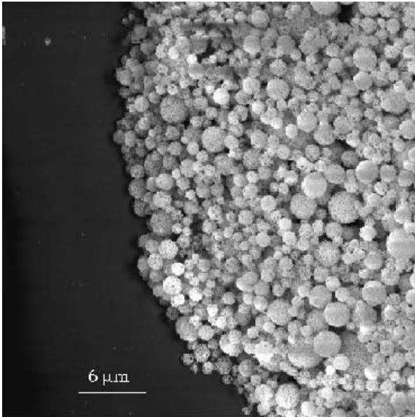
**Figure 7:** Higher magnification view SEM of ink jet printed  $Zn_2SiO_4:Mn$  phosphor powder dots with 90 micron diameters.
