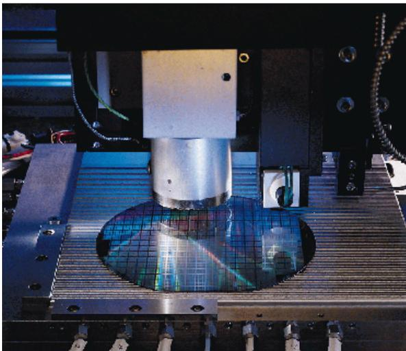
**Figure 3: View of the print head and targeting microscope above an 8" wafer.**
