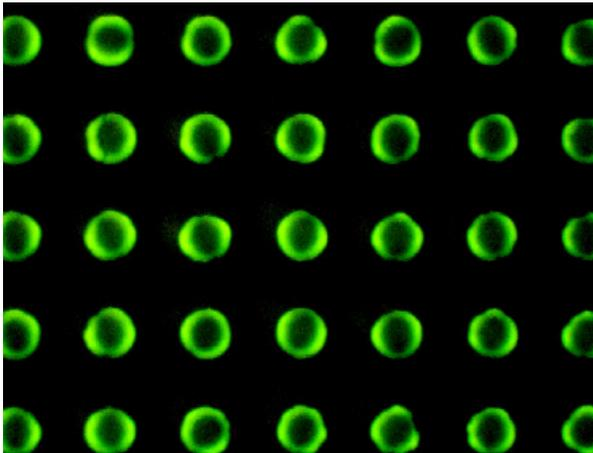
**Figure 10:** Array of printed LEPs in UV illumination.
