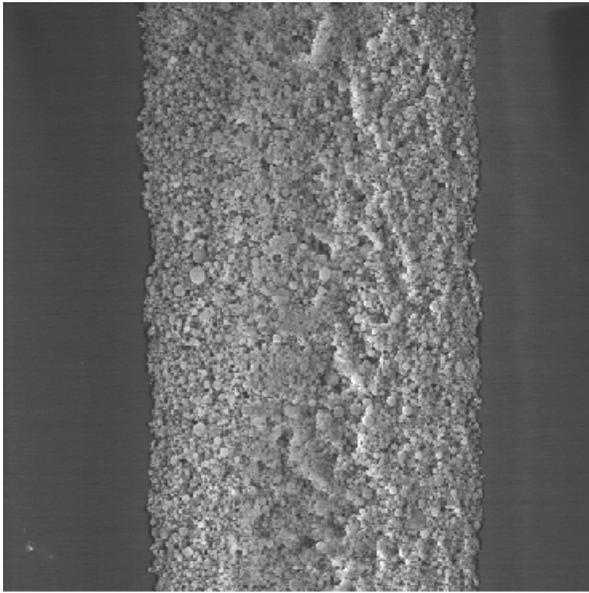
**Figure 9:** Higher Magnification SEM of ink jet printed  $Zn_2SiO_4:Mn$  phosphor powder 90 micron line.
