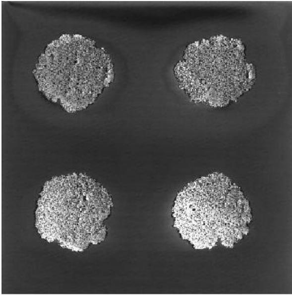
**Figure 6:** Higher magnification view SEM of ink jet printed  $Zn_2SiO_4:Mn$  phosphor powder dots with 90 micron diameters.
