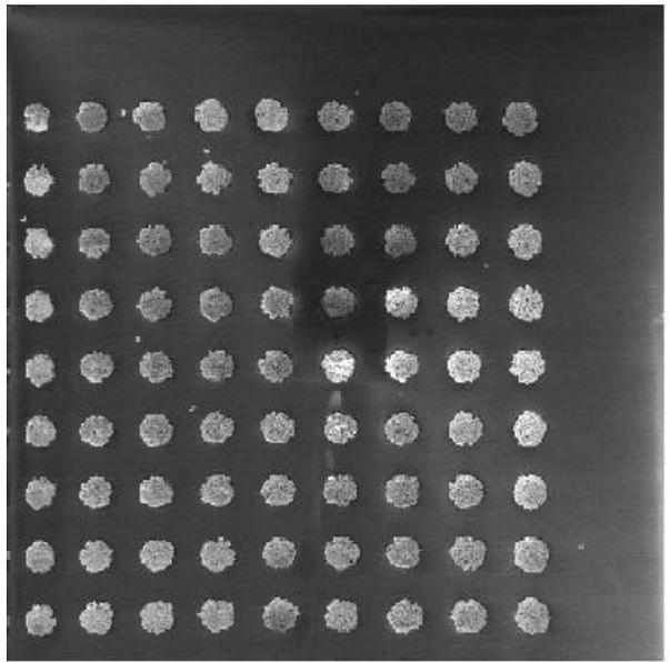
**Figure 5: SEM of ink-jet printed  $Zn_2SiO_4:Mn$  phosphor powder dots with 90 $\mu$ m diameters.**
