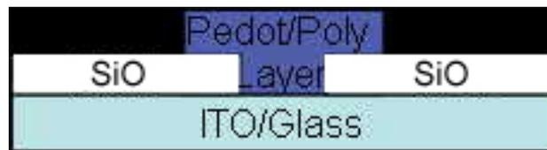
**Figure 10 Cross-section of layered (partial) PV structure.**
