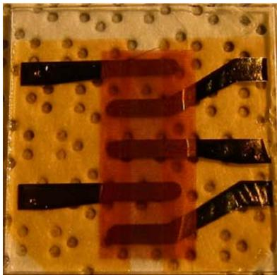
Figure 12 A completed photovoltaic device on ITO/glass.
