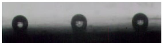
Figure 7. Profile view of 65 :  $m$  diameter hemispherical microlenses printed onto the tips of single-mode fibers within a fiber array (fiber array courtesy of Radiant Research Inc.).
