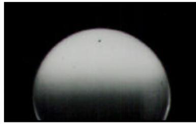
Figure 16. Simulated AGRIN microlens, 300  $\mu\text{m}$  in diameter, printed by depositing fluorescing optical epoxy onto a prior deposition of non-fluorescing epoxy, viewed in profile under UV-irradiation.
