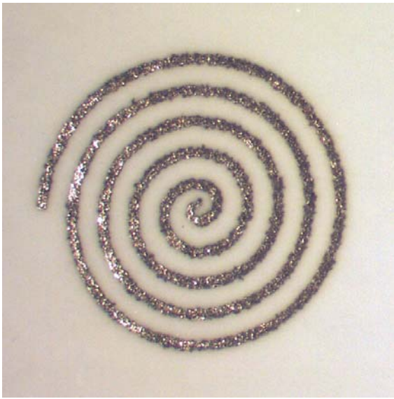
Figure 2: Antennae printed using Cabot's silver ink; 10mm across
