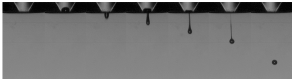
Figure 6. Drop ejection sequence of an organic solvent at 640Hz
