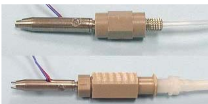
Figure 7. MJ-AT type device with a MINSTAC coupler. Top: MINSTAC 062 couple male to male using a union. Bottom: MINSTAC coupler male to Luer using an adapter
