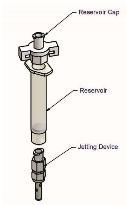
*Figure 5 - MJ-AL-01 device with PH-41 reservoir cartridge*
