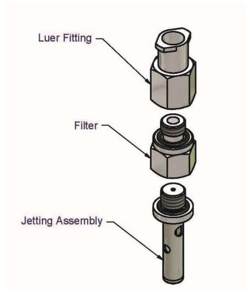
Figure 2 - Components of the MJ-AL-01 device
