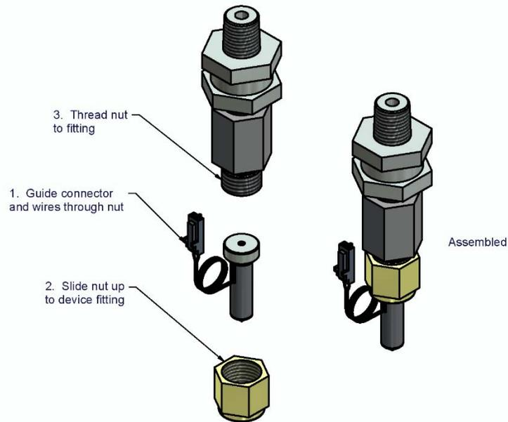
*Figure 4 - Installation sequence*
