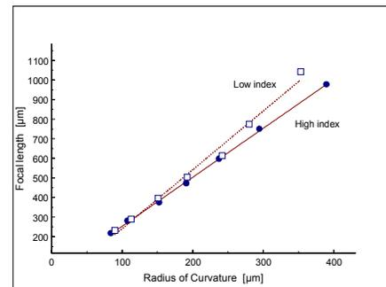
Figure 7: *Focal length vs. radius of curvature for small lenses with different indices of refraction.*
