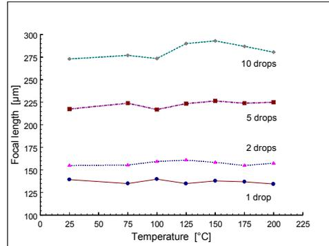
Figure 4: *Focal length vs baking temperature for different lens sizes (numbers of droplets)*
