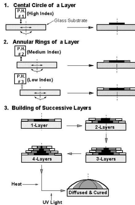
Figure 5: *Process steps for radial GRIN lenses.*
