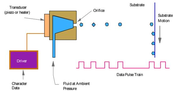
Figure 1: *Principle of drop-on-demand dispensing.*
