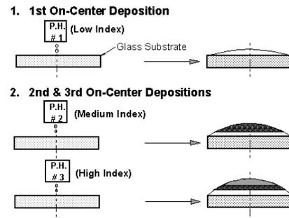
Figure 6: *Printing steps for axial GRIN lenses.*
