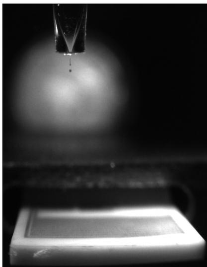
**Figure 7** – Image captured with the CCD camera showing the drop generation under stroboscopic illumination. The generated droplets land on the heater element.
