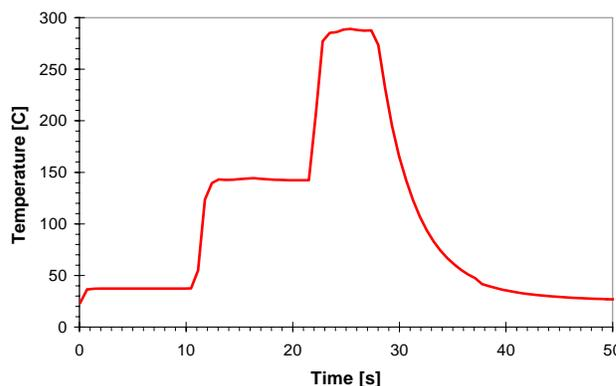
**Figure 11** – Temperature profile measured using a thermocouple in contact with the top surface of the heater. Settings: ramp 1 – 1 second; temperature 1 – 40°C for 10 seconds; ramp 2 – 1 second; temperature 2 – 150°C for 10 seconds; ramp 3 – 1 second; temperature 3 – 300°C for 5 seconds
