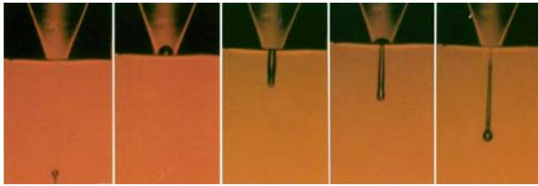
**Figure 1** – Sequence of generation of 50µm droplets (ethylene glycol) at 4kHz
