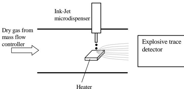
**Figure 2** – Basic components of the vapor generator
