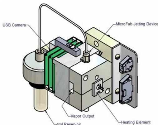
**Figure 5** – Printhead module and its main components
