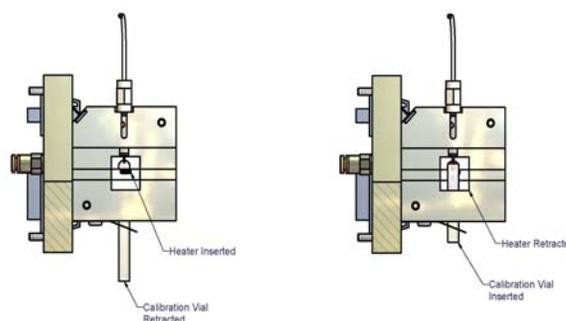
**Figure 6** – Dispenser head shown: left - with the heater in normal operation position; right – with the heater retracted and the collection vial pushed in.
