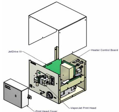
**Figure 4** – Portable vapor generator and its main components
