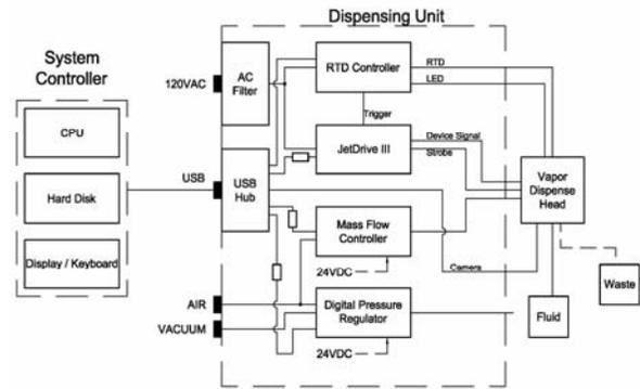
**Figure 3** – Diagram of the vapor generator indicating the main components
