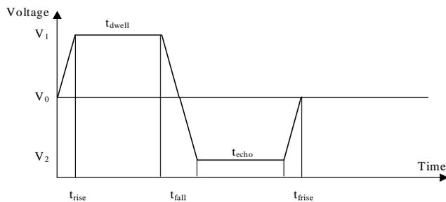
**Figure 8** – Waveform applied to the piezoelectric actuator
