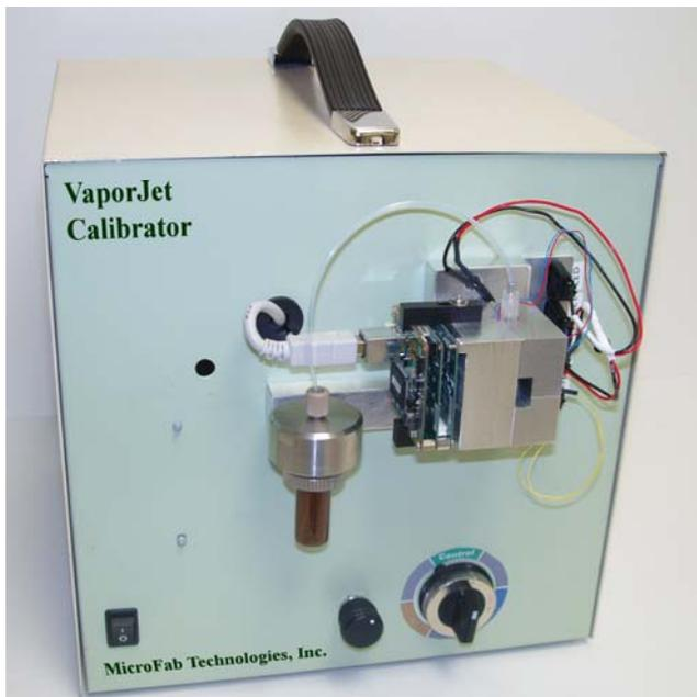
**Figure 10** – Support module (box) and the dispensing module (front of the box)
