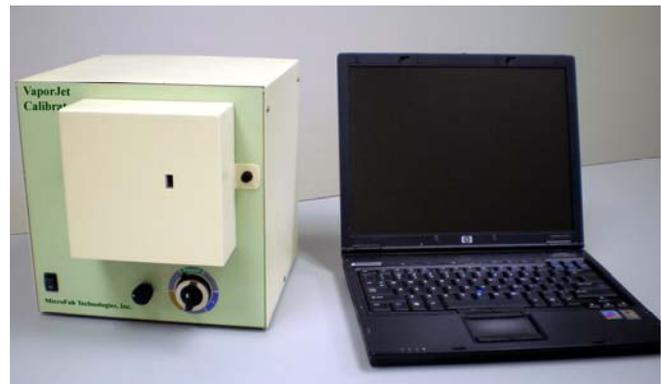
**Figure 9** – Vapor Generator and control laptop
