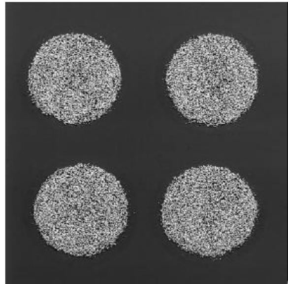
Figure 13: 150µm spots of ferrite particles; MicroJet printed.
