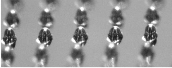
*Figure 5: 100 $\mu$ m diameter solder bumps placed onto 100 $\mu$ m pads on 250 $\mu$ m centers at 400 per second on the MPM Solder Jet feasibility platform.*
