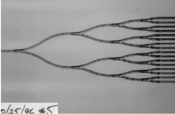
Figure 11: 100µm polymer waveguide / splitter created using MicroJet Technology.
