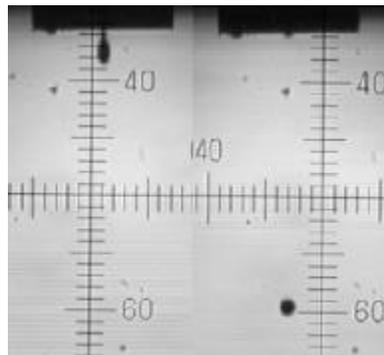
*Figure 3: Drop formation process for a solder at two times during the process. Drop rate is 120 Hz and drop size is 62 $\mu$ m.*
