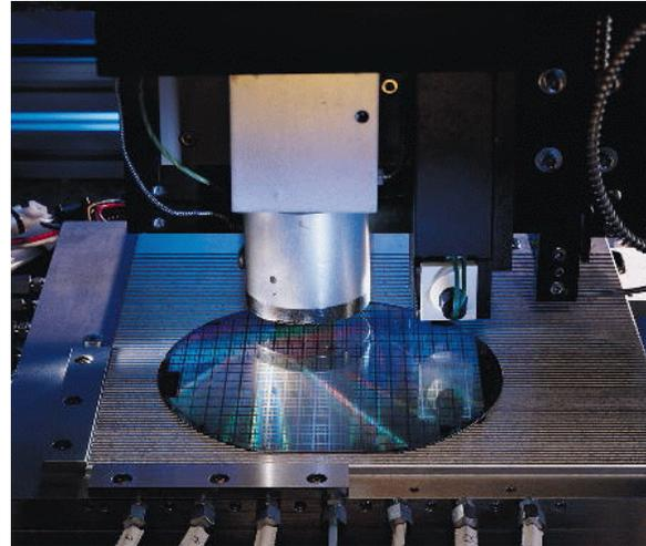
**Figure 2: MicroJet printhead mounted on a platform.**
