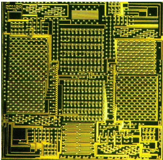
*Figure 6: IC test vehicle with 1440 pads, bumped with 63/37 using MicroJet Technology. Ball size is 70 $\mu$ m.*
