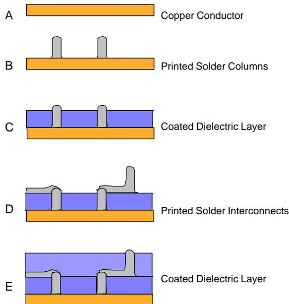
Figure 9: Printed Solder Interconnect Concepts
