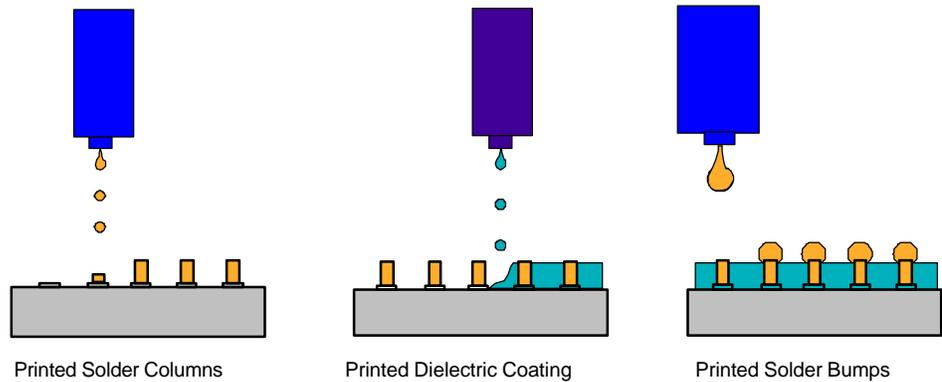
Figure 8: CSP Method of Manufacturing.
