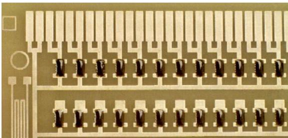
Figure 12: 0402 resistors printed using MicroJet Technology; filled, UV curing epoxy.
