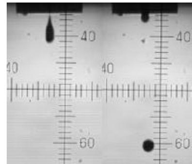
*Figure 4: Drop formation process for same device shown in the previous figure, but using a different drive waveform. Drop rate is 120 Hz and drop size is 106 $\mu$ m.*
