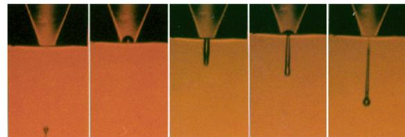
**Figure 1: Demand mode ink-jet device generating 50 $\mu$ m diameter drops at 2kHz.**
