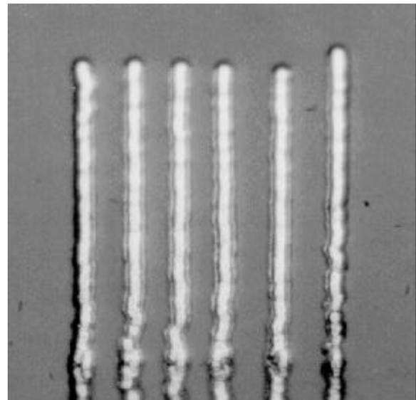
Figure 10: 25µm diameter towers on 50µm centers of 63/37 created using MicroJet Technology.
