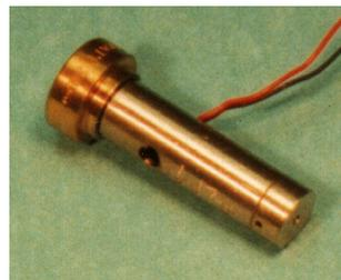
**Figure 7.** Single channel,  $33\text{mm}$  long, drop-on-demand device for dispensing at temperatures to  $240^\circ\text{C}$ .
